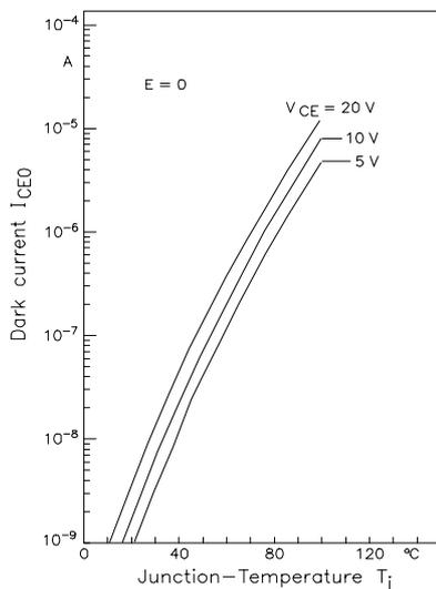
Figure 16. Temperature-dependence of the collector dark current
