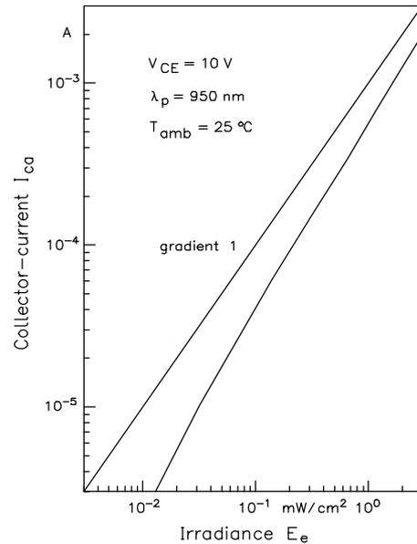
Figure 8. Sensitivity of the reflex sensors' detector
