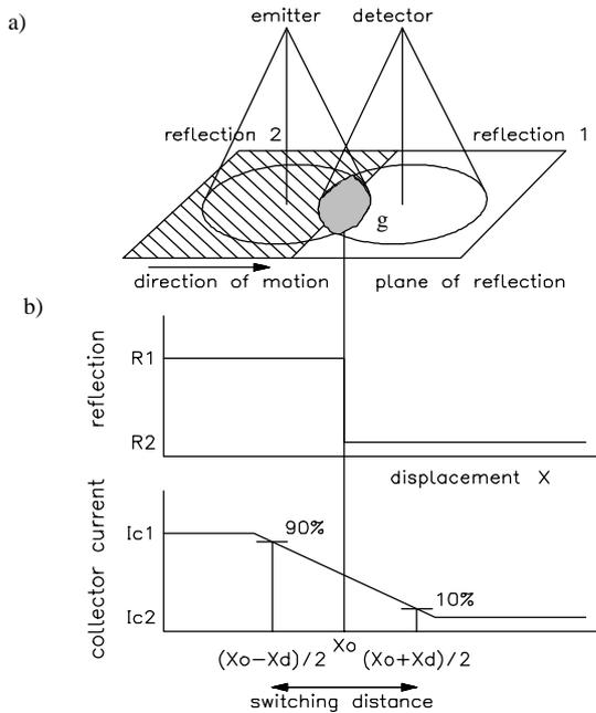
Figure 13. Abrupt reflection change with associated  $I_c$  curve
