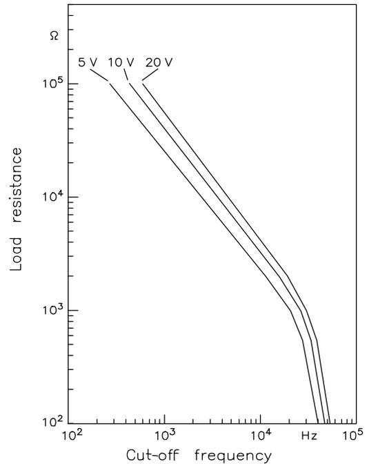
Figure 11. Cut-off frequency,  $f_c$
