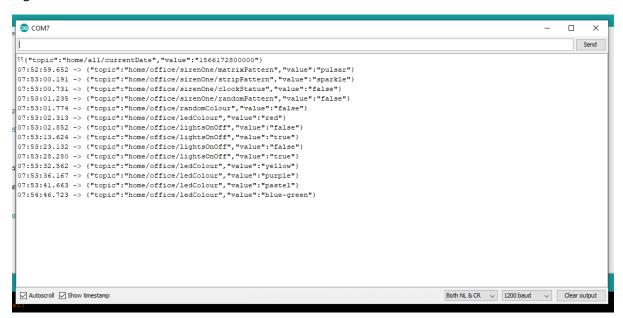
So now I can see the NodeMCU connected to the network and receiving messages from my MQTT server, and sending this JSON over the Serial Port.
