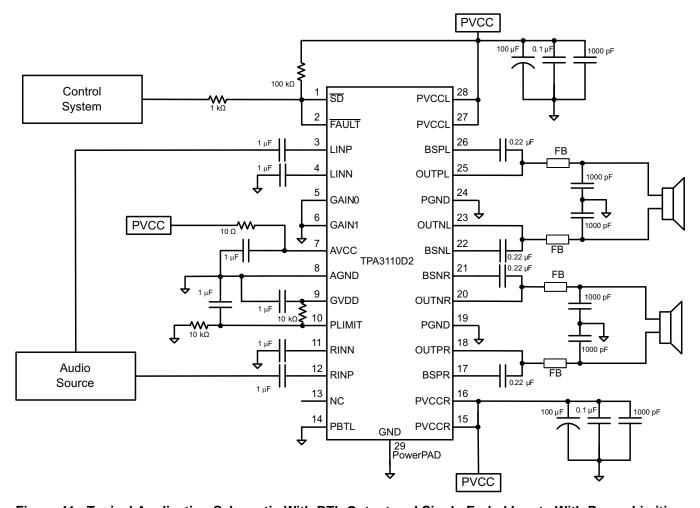
Figure 41. Typical Application Schematic With BTL Output and Single-Ended Inputs With Power Limiting
