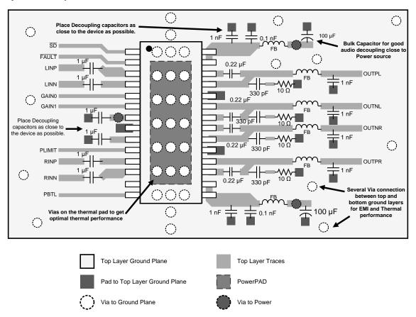
Figure 47. TPA3110D2 PCB Layout
