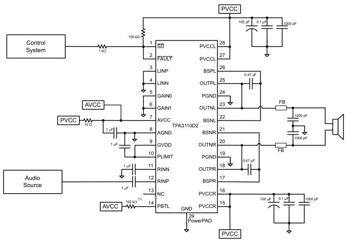
(1)  $100 \text{ k}\Omega$  resistor is needed if the PVCC slew rate is more than 10 V/ms.
