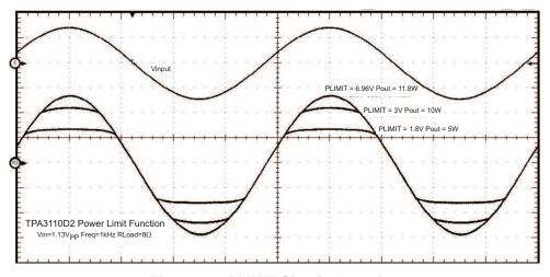
Figure 40. PLIMIT Circuit Operation
