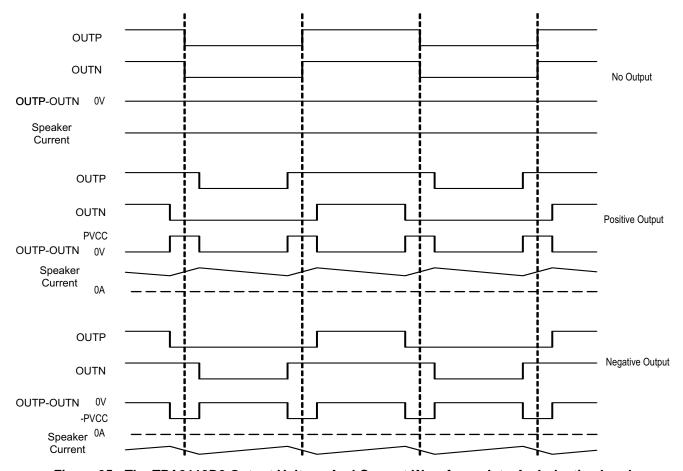
Figure 35. The TPA3110D2 Output Voltage And Current Waveforms Into An Inductive Load
