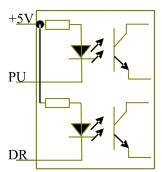
Figure: 6.1-2 Three Inputs, Common-anode Input Signal of Driver
