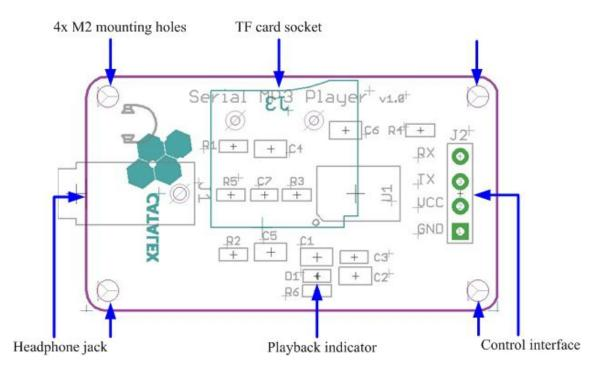
**Control interface:** It is UART TTL interface. A total of four pins (GND, VCC, TX, RX), GND to ground, VCC is the power supply, TX is the TX pin of the MP3 chip, RX is the RX pin of the MP3 chip.
