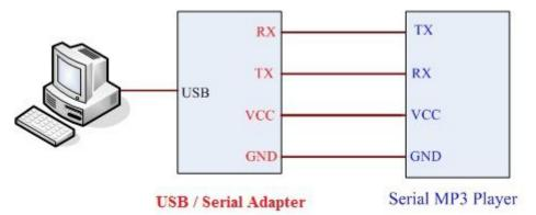
(2) After the connection is completed, open <u>the sscom32 serial tool</u> that you can down load from catalex net disk to send commands. About the specific commands, please refer to 4.1.1 part.
