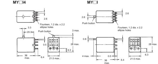
Note: 1. Mount the relay with a socket.
