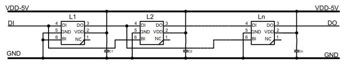
Remarks: Cn is external filter capacitor, its value of 100NF.
