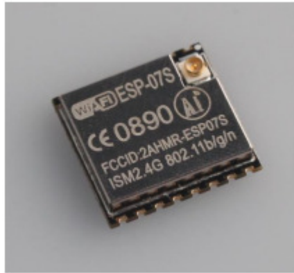
Figure 3 Top View of ESP-07s WiFi Module
