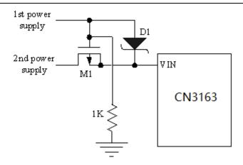
Figure 6 Combining 2 Input Power Supply
