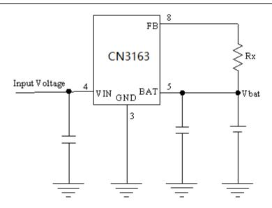
Figure 5 Adjusting Regulation Voltage in Constant Voltage Mode
