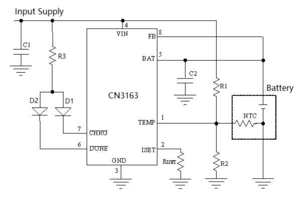
Figure 7 Monitoring Battery Temperature
