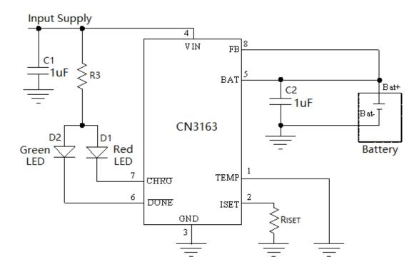
Figure 1 Typical Application Circuit(Constant Voltage Level 4.2V)
