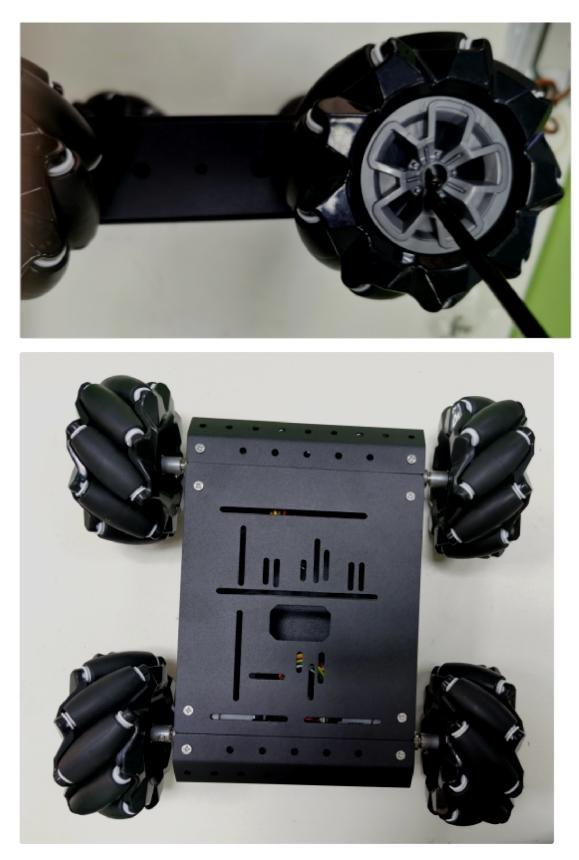
Special note: If you use the program we provide, the direction of the wheel should be consistent with the picture.
