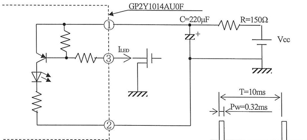
(\*4) Sampling timing of output pulse
